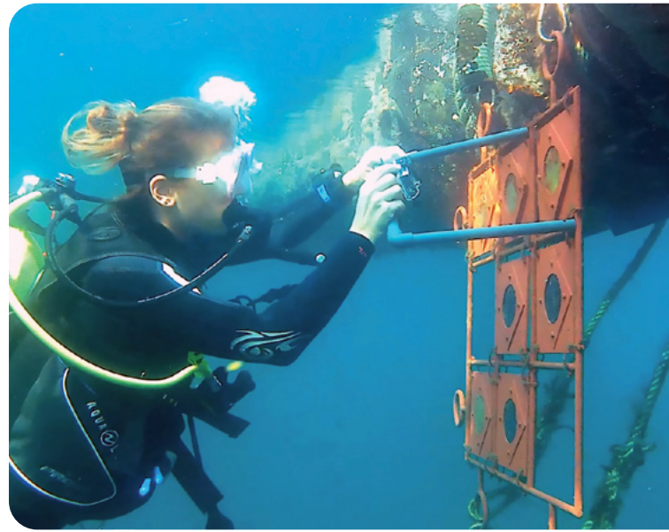
Biofouling test in the Malta sea of the AIRCOAT samples.
