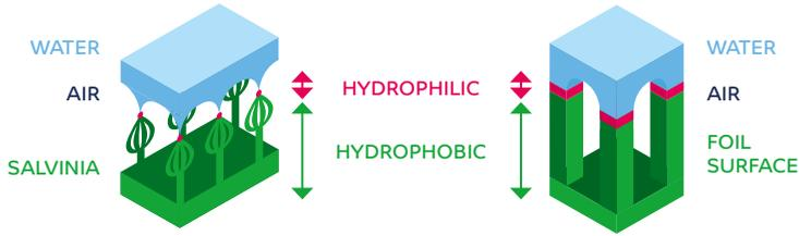
1. Development of the surface/foil implementing the Salvinia effect, that is able to trap a layer of air when submerged in water.
