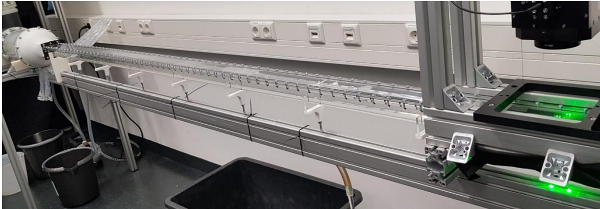
Fig.7: Image of the constructed the LDA flow tank with major parts and flow paths. The red arrow indicates main flow direction (top left) and detailed rendering of the nozzle with 3D-printed connectors and adjacent parts (top right).
