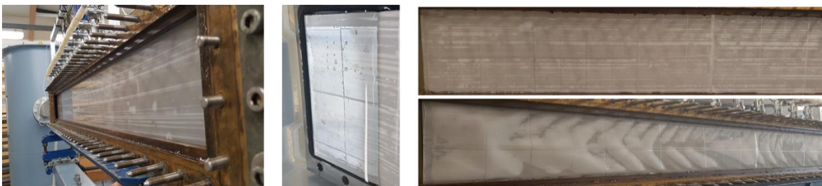
Fig.8: Images of the friction tank experiments at SVA. Left: Flat control installed in the friction tank. Middle: AIRCOAT foil submerged in water after experiments done at 6 m/s – note the clearly visible, silvery shining air layer. Right: AIRCOAT foil installed in the friction tank before (top) and after the last experiment with maximum velocity of 17 m/s (below).
